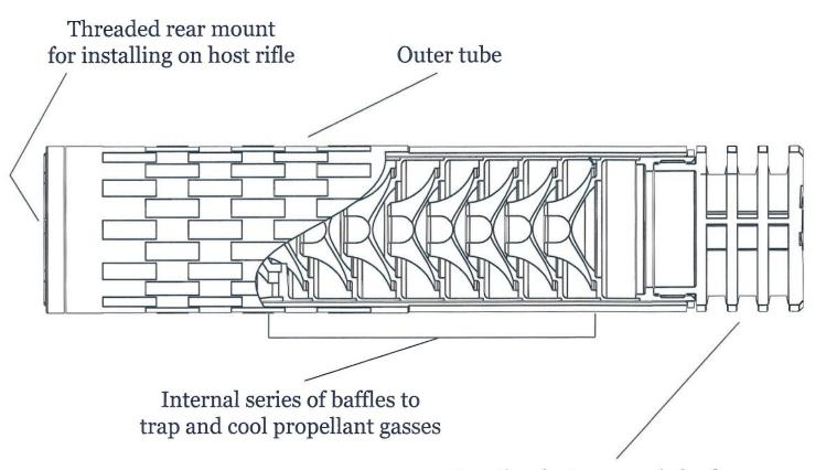
Recoil reducing muzzle brake incorporated into front end cap
